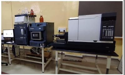
operational pressure based on their physicochemical properties. Individual components are then ionised and separated based on the mass-to-charge ratio (m/z) in the mass analyser, creating a spectrum that provides the elemental signature of the sample.
