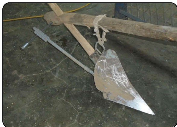
Fig. 2 : Improved animal-drawn moldboard plow (left side) and farmers taking training on how to use the implement (right side) at Melkassa Agricultural Research Center (Source: Unpublished 2018 progress report)
