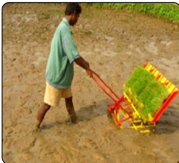
Fig. 10 : Manually operated, hand-cranked rice transplanter walking backward type (left) and walking forward type (right)
