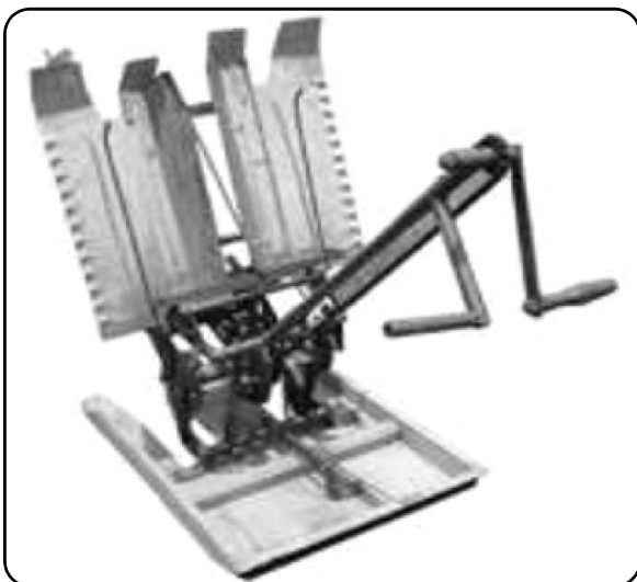
Fig. 10 : Manually operated, hand-cranked rice transplanter walking backward type (left) and walking forward type (right)
