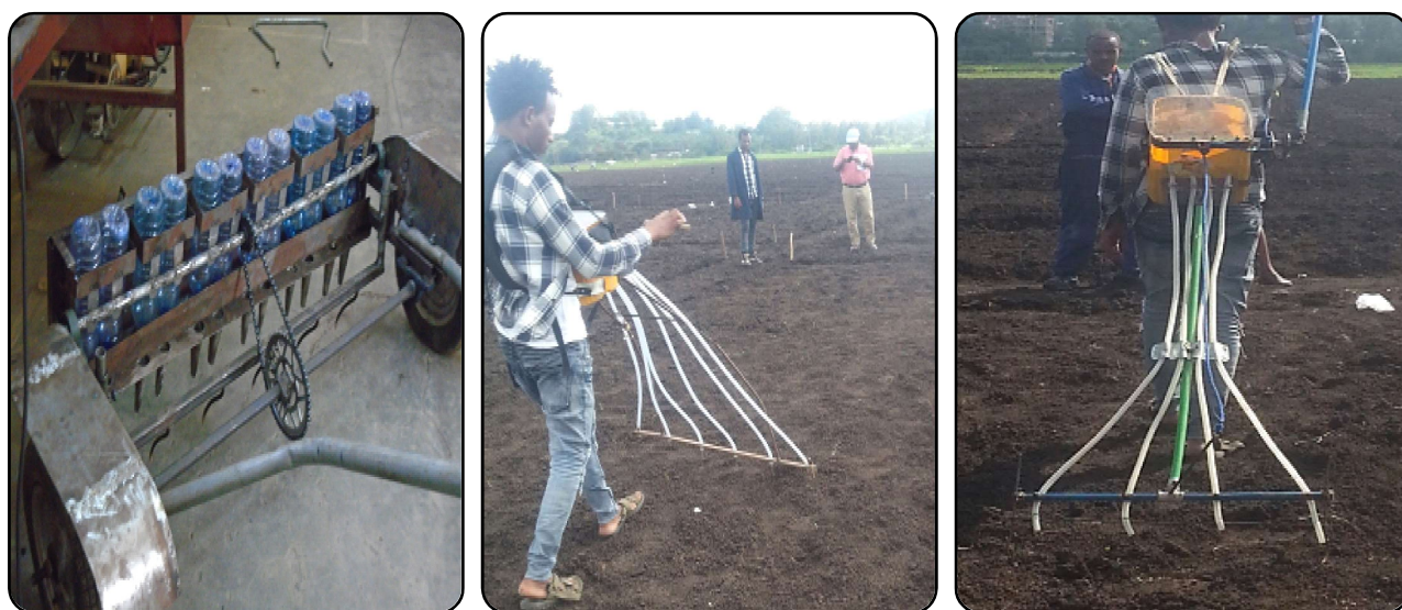
Fig. 4 : Different prototypes of teff seed drills developed at Melkassa Agricultural Research Center: Manually operated, 12-row plastic bottle teff seed drill (left side), Front pack scoop type six row teff seeder(middle), Backpack scoop type six-row teff seeder(right side)
